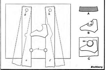
Fig. 5. Simple Design of Shaving or Trimming Die
